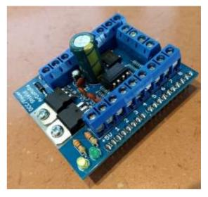
**Option 2**: Power supply using the power components on the board. Connect an AC or DC power supply to the power terminals. You will then have 5V available at 5V connector.
